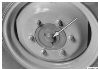
Left and right wheel hubs, R-WD only Unscrew lid, fill with lubricant.
